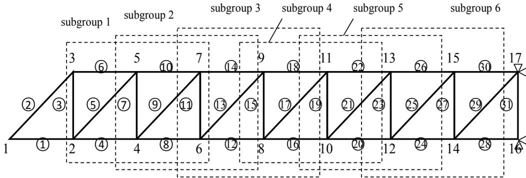
Figure 1. The planar beam-like truss model and the formed subgroups
