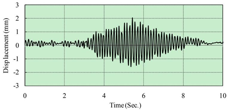
Measured displacement time history of the girder bridge in dynamic load test
