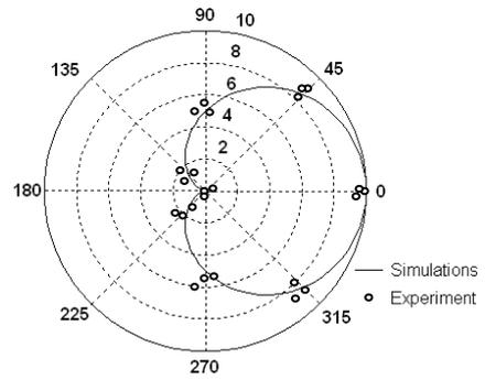
Distribution of circumferential temperature difference of the suspender (unit: °C)
