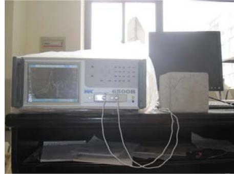
PZT impedance test of concrete cube
