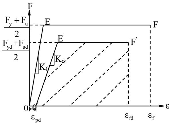
Bilinear approximation of proposed damage indicator for cable wires
