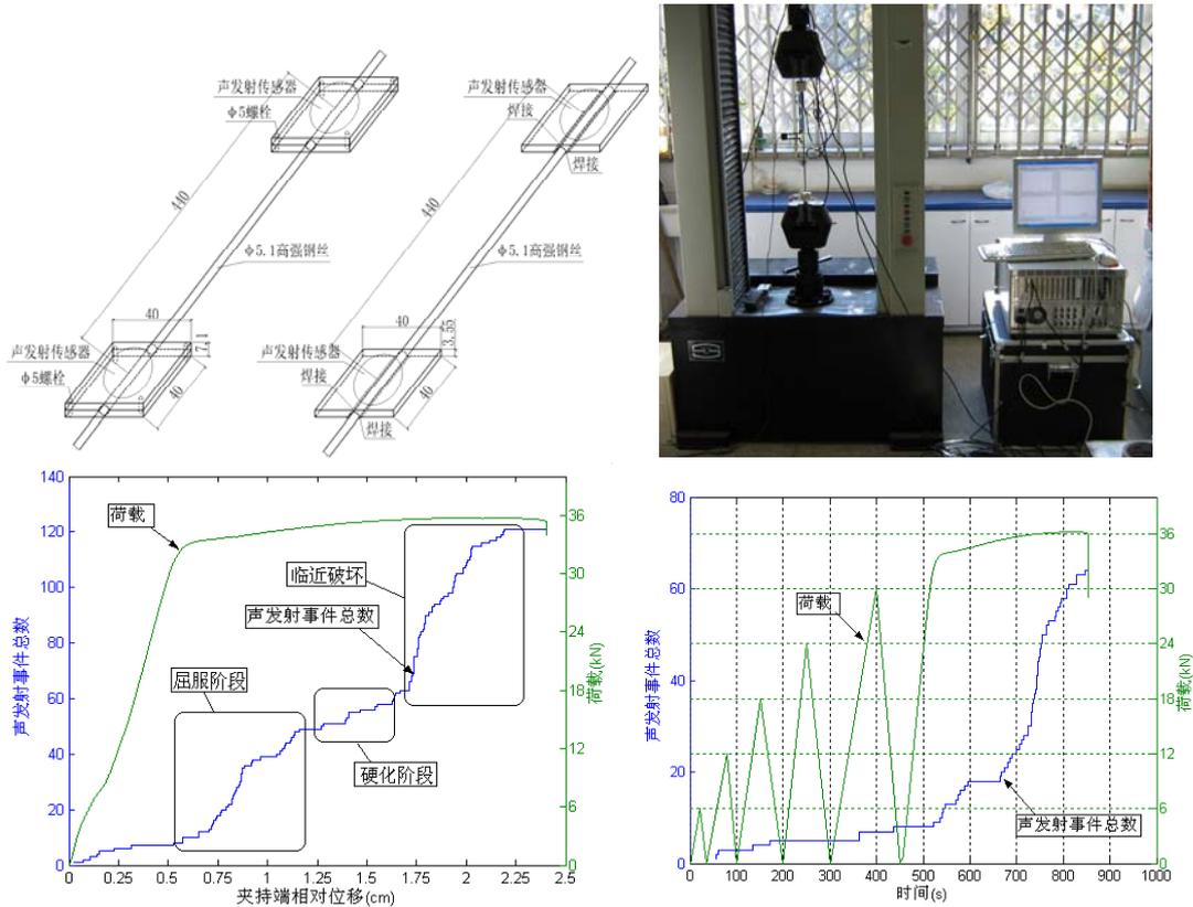
AE experimental setup and test results for steel wires in cyclic axial loading.
