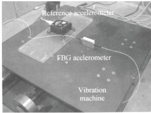
Calibration test of FBG accelerometer
