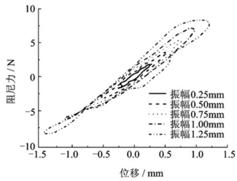
Tested hysteretic curve of a single viscous damper
