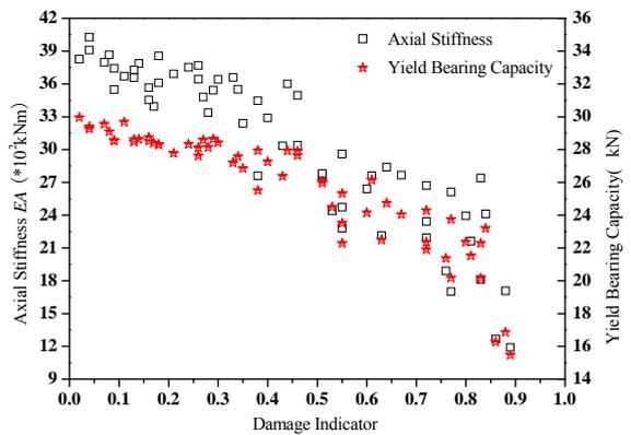
Degradation of wires' mechanical properties with damage indicator
