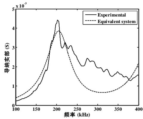
The measured and re-constructed admittance spectrum
