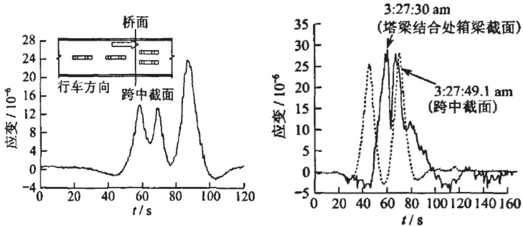
FBG strain measurement on the main navigation channel bridge of Donghai Bridge
