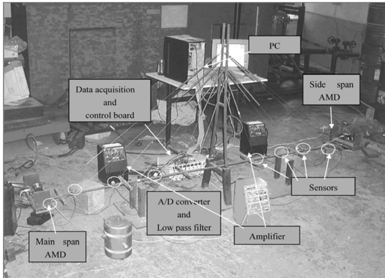
Experimental setup of the AMD equipped cable-stayed bridge in construction
