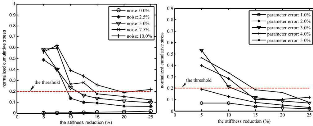
Modeling error and noise effect on damage diagnosis accuracy
