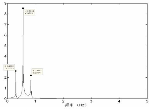
On-site measurement of cable dynamic deformation on Sutong Bridge
