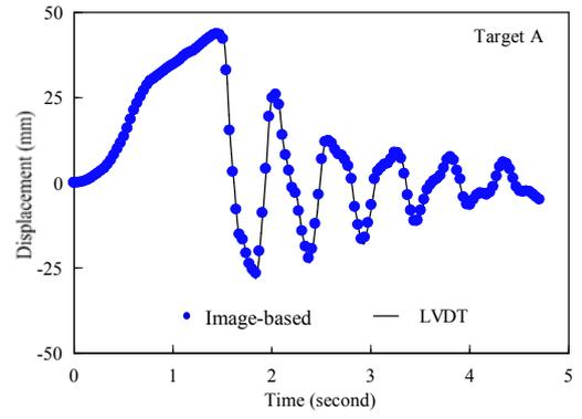
Measured response in wind tunnel test
