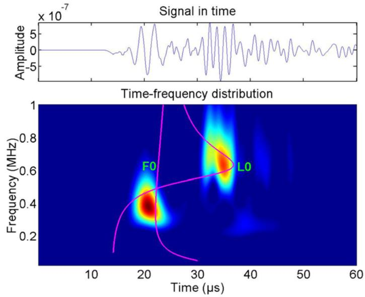
The simulated wave propagation measurement in seven-wire strand.
