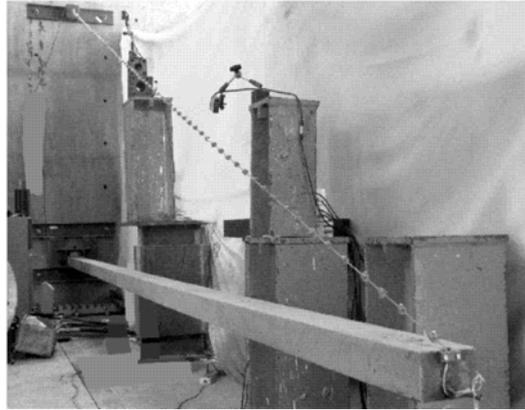
The girder-cable-damper coupled vibration system and test setup
