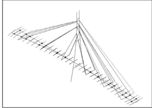
The symmetric and anti-symmetric modes with the same resonant frequencies
