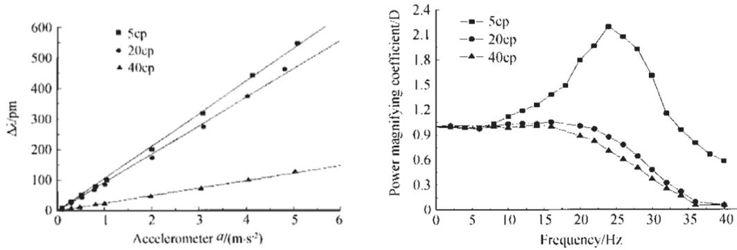
Sensitivity, linearity, and amplitude-frequency test of prototype FBG accelerometer
