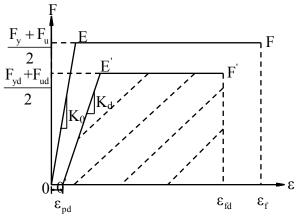
$\begin{array}{ccc} \epsilon_{pd} & \epsilon_{f} \\ \text{Bilinear approximation of proposed damage} \\ \text{indicator for cable wires} \end{array}$
