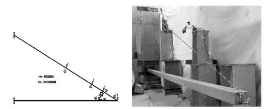
The girder-cable-damper coupled vibration system and test setup
