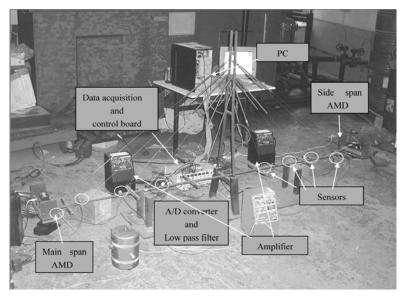
Experimental setup of the AMD equipped cable-stayed bridge in construction
