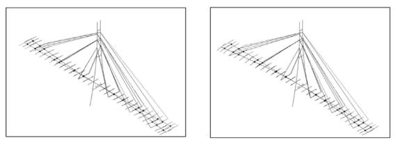
The symmetric and anti-symmetric modes with the same resonant frequencies
