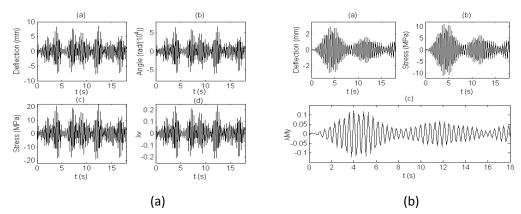
Dynamic response of short suspender with (a) vertical vibration; (b) longitudinal vibration.
