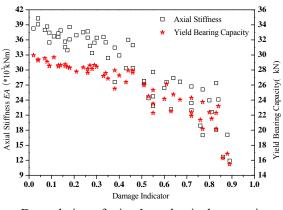
Degradation of wires' mechanical properties with damage indicator
