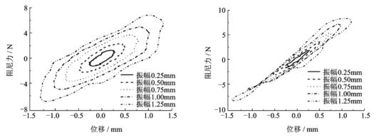
Tested hysteristics curve of a single viscous damper
