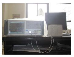
PZT impedance test of concrete cube
