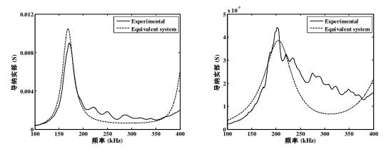
The measured and re-constructed admittance spectrum
