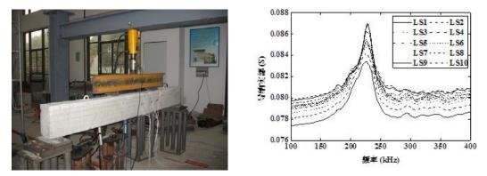
Loading tests of RC beam and the PZT admittance measurement
