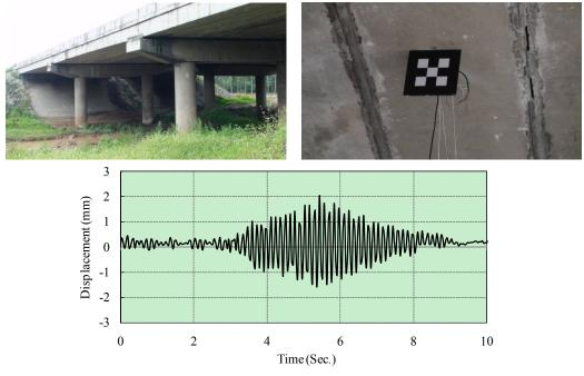
Measured displacement time history of the girder bridge in dynamic load test
