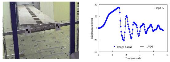
Measured response in wind tunnel test
