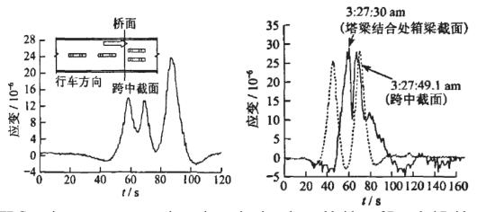
FBG strain measurement on the main navigation channel bridge of Donghai Bridge
