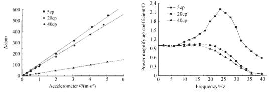
Sensitivity, linearity, and amplitude-frequency test of prototype FBG accelerometer
