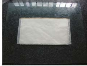
Fig. 2. Lay down glass fiber fabric and release fabric.
