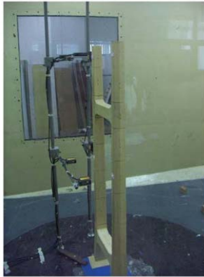
Fig. 3. (Color online) The aeroelastic model of the pylon of the Minpu Bridge.
