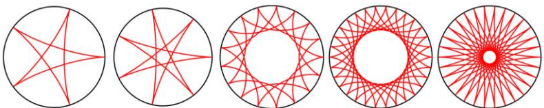
Figure 4: Hypocycloid for rational values of a/b = \frac{5}{3}, \frac{7}{3}, \frac{17}{4}, \frac{30}{7}, and \frac{30}{13} .
